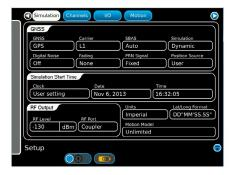
The Setup page is partitioned via a tab selection scheme to allow control for Simulation, Almanac, Channels and I/O.
